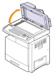
**2** Place the original **face down** on the scanner glass and align it with the registration guide at the top left corner of the glass.
